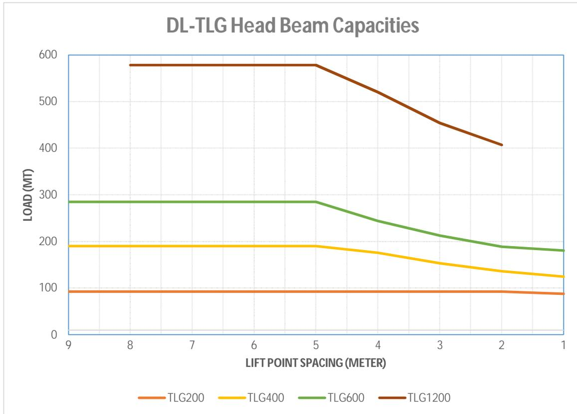
The above graph is plotted considering maximum span = 11.3m, Load centre offset = 0m and 1<sup>st</sup> stage of the ram. For complete lifting arrangement and duty charts please refer the respective telescopic lifting gantry drawing.
